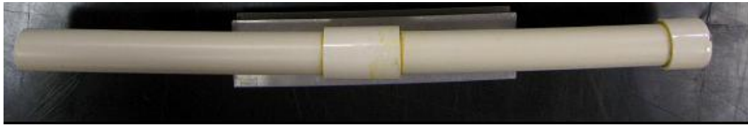
Figure 3. CPVC test pipe with fitting
