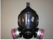
**Respiratory Protection:** A NIOSH-approved air purifying respirator (APR) with combination organic vapor/particulate (P100) cartridges, or a supplied air respirator (SAR) should be used as noted below. Respirators should be used and maintained in accordance with your
